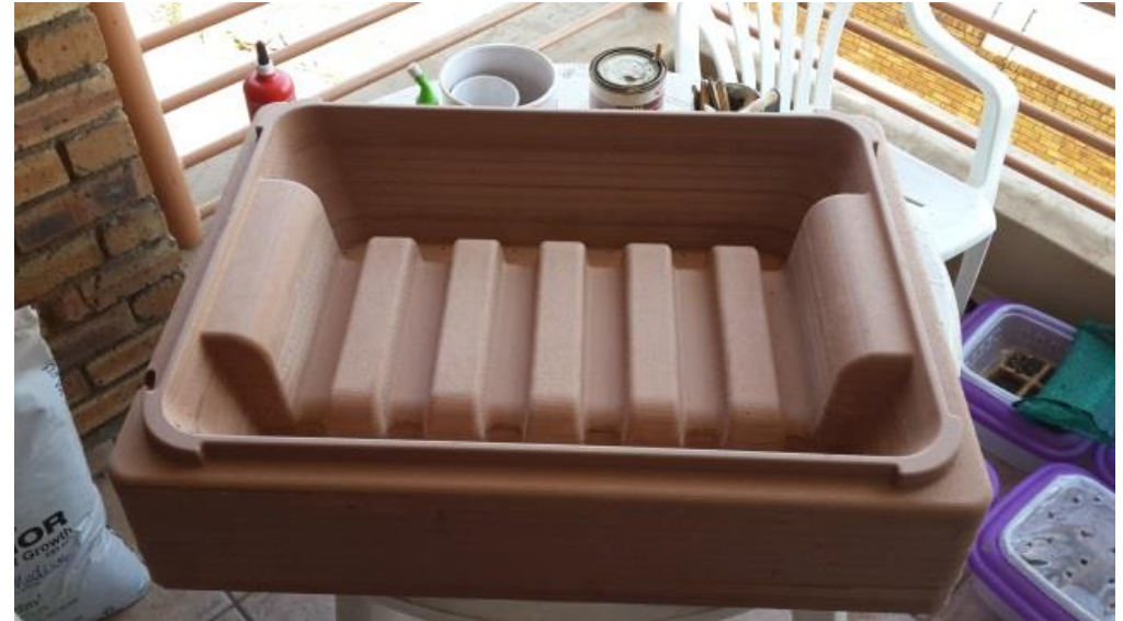
Figure 29: Mould made out of wood for vacuum forming
