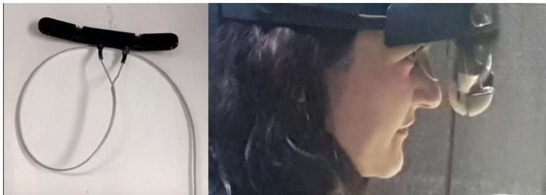
Figure 4: The SMA actuator set into the HoloLens 2 visor.
